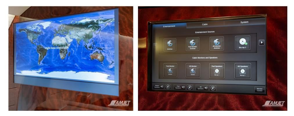
THE HD-CAPABLE VENUE CMS FEATURES BOTH TOUCHSCREEN AND IPAD WIRELESS CONTROL OF ALL CABIN SYSTEMS. IPAD SIDE-LEDGE MOUNTS ARE INSTALLED IN THE FLIGHT DECK TO ALLOW PILOTS TO CONVENIENTLY AND SIMULTANEOUSLY CHARGE AND ACCESS INFORMATION ON THEIR IPADS. SIDE-LEDGE IPAD OR ANDROID MOUNTS ARE INSTALLED AT SIX (6) MAIN CABIN CHAIRS. FORWARD AND AFT 26 INCH CABIN BULKHEAD MONITORS. AIRSHOW AND BLU-RAY.
