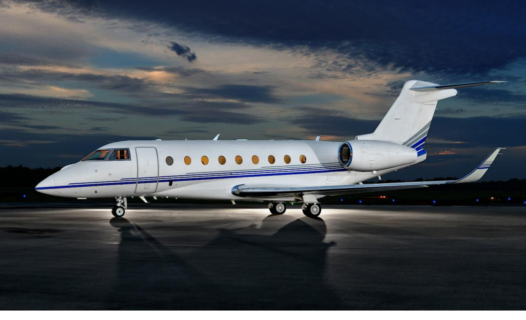
The G280's wing was engineered along the lines of the Gulfstream G550, one of the most versatile aircraft flying today. Because of the exceptional design, the G280 wing needs no leading-edge devices to aid low-speed maneuverability. Instead, subtle contours along a highly swept, smooth wing reduce drag and enhance lift.
