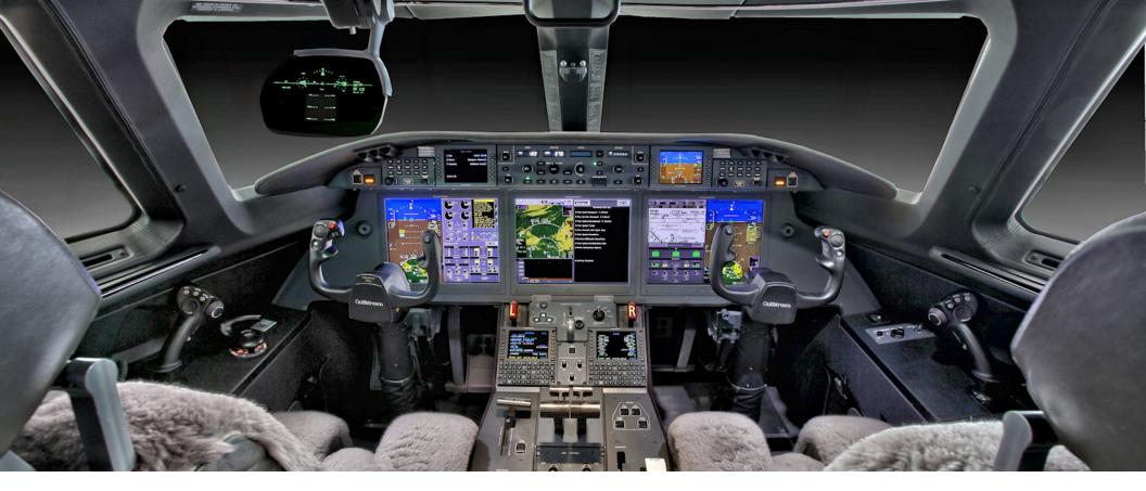
The PlaneView280 flight deck incorporates state-of-the-art flight and navigation systems while autothrottle and autobraking set new standards for aircraft control and handling. In addition, each of these aircraft are equipped with Heads-Up Device (HUD), Enhanced Vision System (EVS), and Synthetic Vision, delivering unparalleled situational awareness and safety to cockpit operations.
