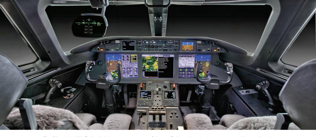
The PlaneView280 flight deck incorporates state-of-the-art flight and navigation systems while autothrottle and autobraking set new standards for aircraft control and handling. In addition, this G280 is equipped with Heads-Up Device (HUD), Enhanced Vision System (EVS), and Synthetic Vision, delivering unparalleled situational awareness and safety to cockpit operations.
